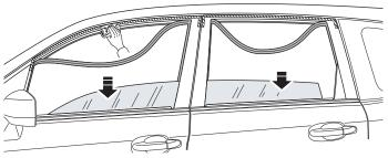
Install clips (5) onto side window deflectors as shown.
